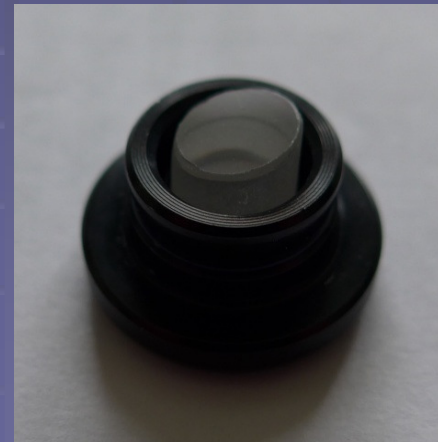
Modified 200 l/mm Grism (Made using the Star Analyser 200 master grating)
