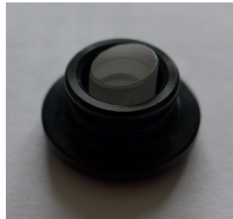
Modified 200 l/mm Grism (Made using the Star Analyser 200 master grating)
